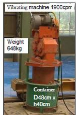
Photo 11- VC test with a large-size container
