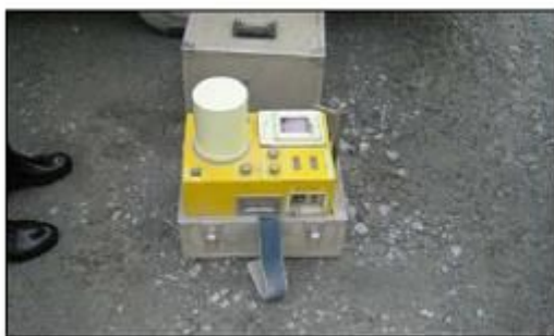
Photo 25- Concrete density measuring by RI meter
