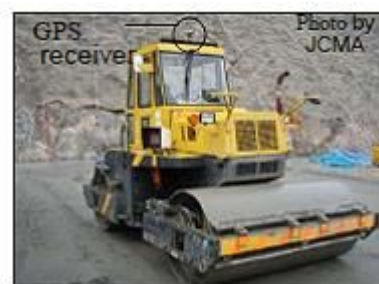
Photo 29- Vibratory roller SD451 with IT, Kasegawa dam
