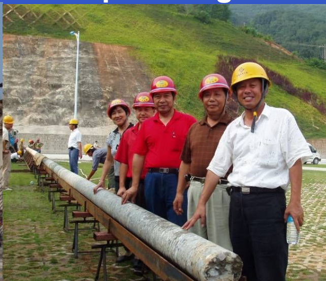
14.3m long RCC core extracting from Jinghong Dam
